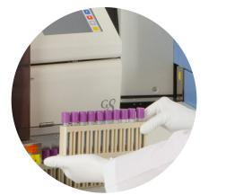
A dedicated holding area allows for extra racks waiting to be sampled to form a queue and reduces the possibility of any back-up at the instrument. This allows for a smooth flow of samples to the G8. While samples are in the holding area, you can continuously load or remove tubes as needed.
